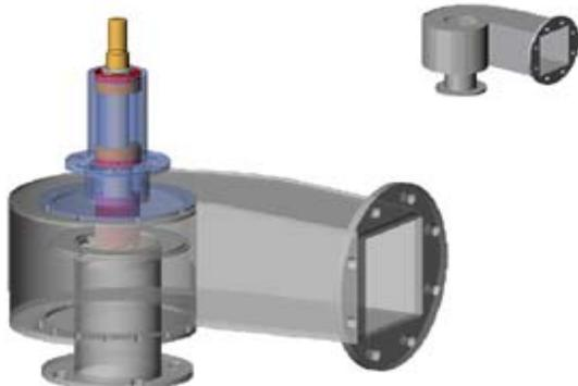
NHE has recently developed the volute cased propeller turbine – which has improved efficiencies to over 73% from the 55% to 60% efficiencies recorded for the open flume designed propeller turbines. A typical 1.2kW propeller turbine requires a flow of 85 litres/s and a height drop of 3.3 metres.
