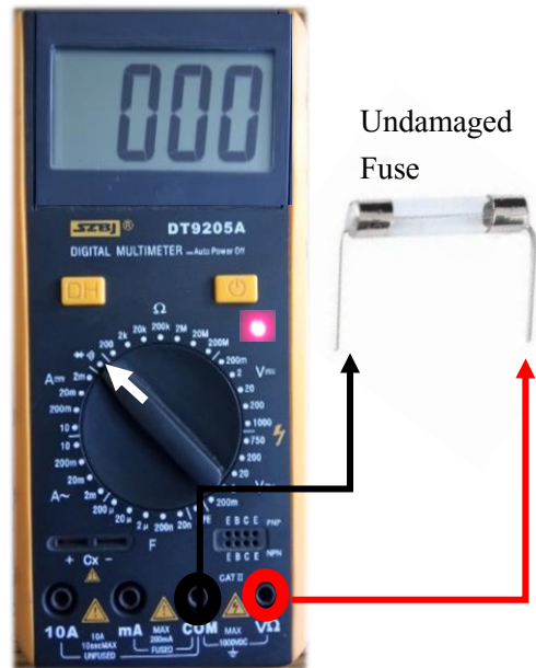
Figure 25: Undamaged fuse indicating a short circuit
