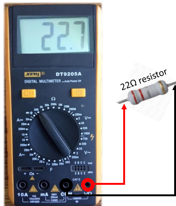
Figure 36: Measurement of resistance using a multimeter
