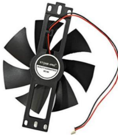
Figure 5: Fan used inside Induction Stove
