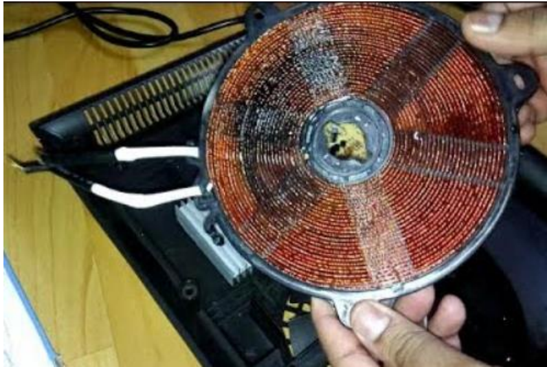
Figure 34: Burnt Induction Coil
