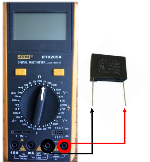
Figure 44: Testing of capacitor using resistance method
