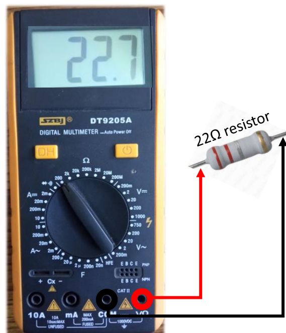
Figure 46: Measurement of resistance using a multimeter
